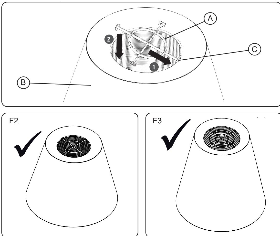
Apply the protective grid (A) to the diffuser (B) as follows:
